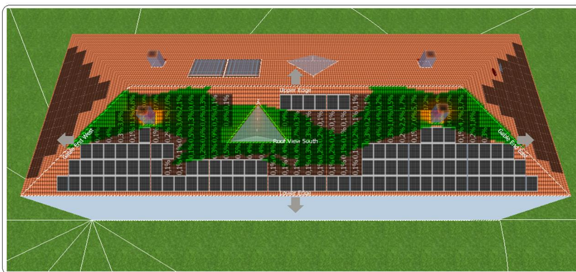
Figure 7. Shadowing analysis of objects on the roof of the solar energy plant
